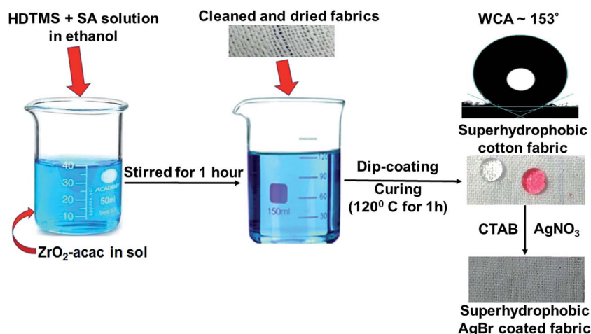
Fig. 1 Schematic representation of the fabrication of superhydrophobic fabric via dip coating approach.
